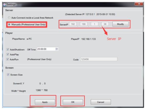
Fixed an IP in pc which install the server software. Fill in the server IP and click apply.
